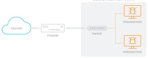
A best practice is to segment the LAN into smaller subnets using zones or VLANs and then connecting these together through the firewall to enable the application of anti-malware and IPS protection between segments. This can effectively identify and block threats attempting to move laterally on the network.
